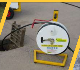
DRAIN JETTING REELS
